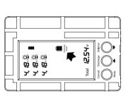
2. Disharge Mode show, SS symbol start flash, it means start discharge mode.
